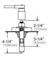
Tighten nut with Torque wrench to 85 ft.-lbs (115nm).
