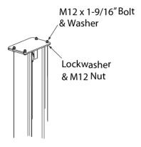
Position the columns facing each other 134-5/8" (3419mm) outside base plates. Square the columns by measuring diagonally from corner points on base plates (within 1/4" (6mm)).
