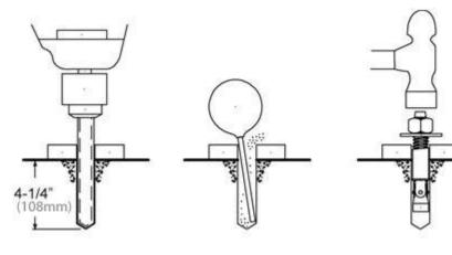
Drill holes using 3/4" (19mm) carbide Tipped masonry drill bit per ANSI standard B94.12.1977
